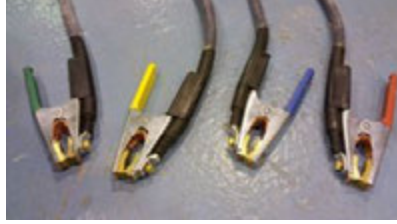
Insulated cable with high current resistance
